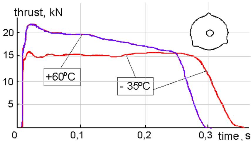
Fig. 4. Thrust vs. time diagram recorded in full-scale test of SC-H0-V0 ejection seat loaded with type C charges, at temperature +60°C and -35°C. The mark at top right corner indicates the shape of a propelling charge cross-section
