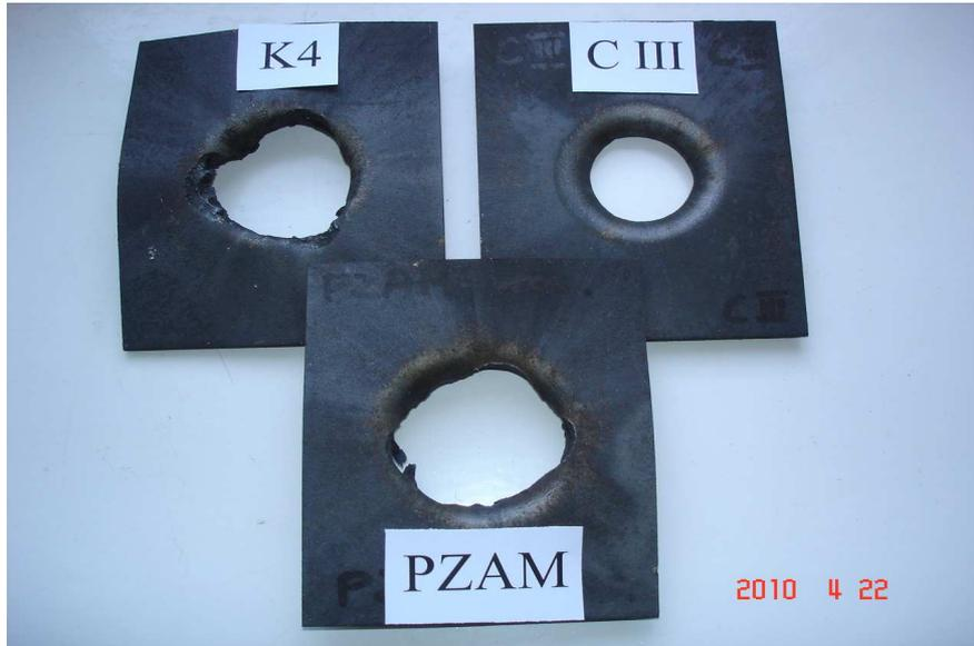
Fig. 7. Picture of steel plates perforated by detonation of propelling charges under study
