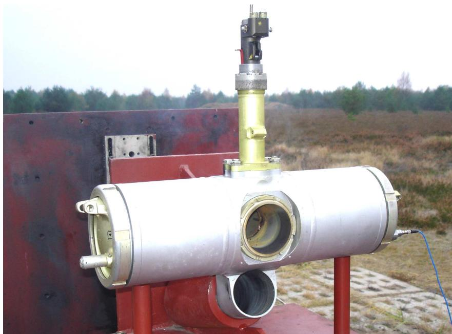
Fig. 5. View of the ballistic stand with a rocket motor of K36DM ejection seat prepared to test. Coaxial cable seen at right is connected with a pressure gauge fixed to the right bottom. Gauge of the thrust is placed behind the rocket motor, along with the axis of the nozzle, seen at the center of the picture.
