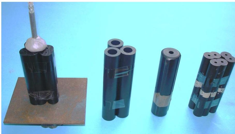
Fig. 7. Picture of propelling charge ready to test of the ability to detonation (left) and other propelling charges tested in the work: PZM, C and PZAM
