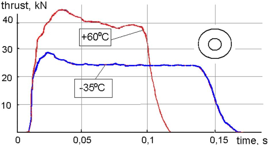
Fig. 3. Thrust vs. time diagram recorded in full-scale test of KM1M ejection seat loaded with charges of modernized shape (PZMM) at temperature  $+60^{\circ}\text{C}$  and  $-35^{\circ}\text{C}$ . The mark at top right corner indicates the shape of a propelling charge cross-section
