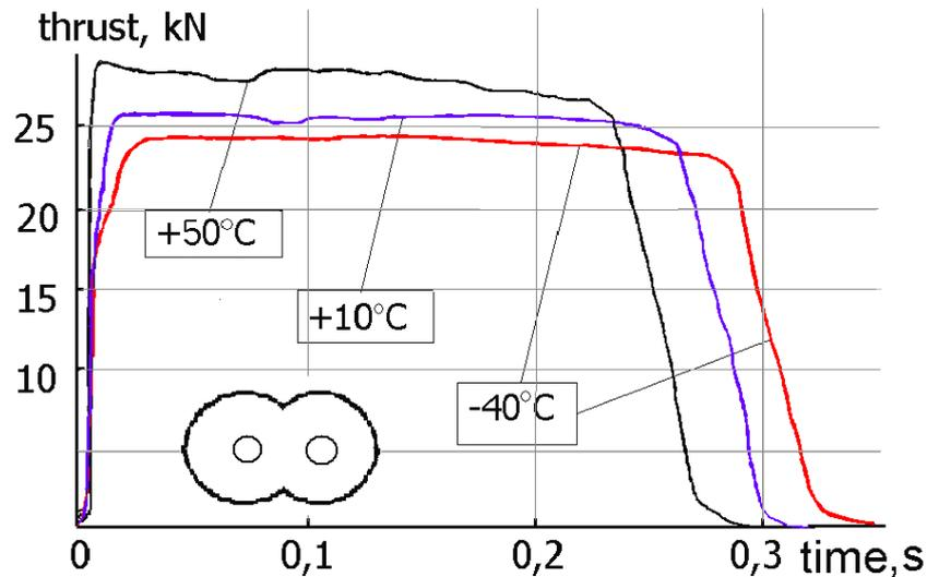
Fig. 6. Thrust vs. time diagram recorded in full-scale test of K36DM ejection seat loaded with PZAM charges, at temperature +50°C, +10°C and -40°C. The mark at left bottom right corner indicates the shape of a propelling charge cross-section
