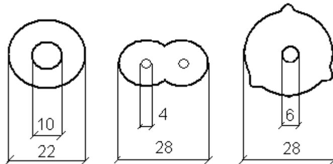
*Fig. 1. Cross-sections of propelling charges used in rocket motors of ejection seats: KM1M, K36DM and SC-HV-00 correspondingly*
