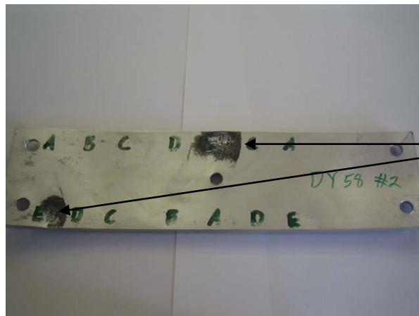
Witness plate for failure diameter test
