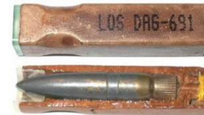
Final G11 Cartridge Configuration (Telescoped)
