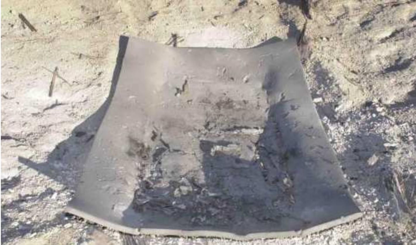
The largest piece of warhead case recovered was 6.5 lb (found 1165 ft down range). It was an asymmetric nose fragment, believed to be from the acceptor. Appearance of all recovered fragments was consistent with at least a Type II (Partial Detonation) reaction.
