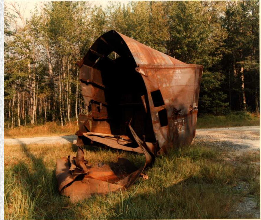
Structural failure from propellant burn
