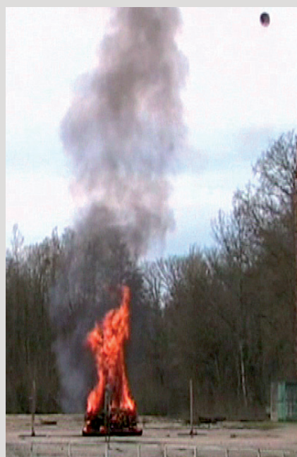
Picture caption: UN External Fire propelled lid in the upper right corner
